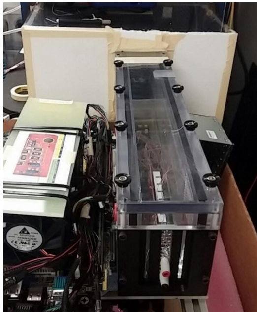
Figure C-6. Actual Thermal Level Test Fixture Set-up
